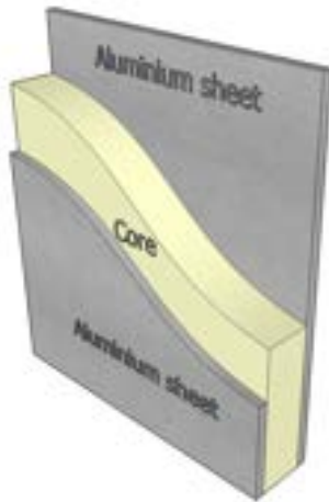
Aluminium insulated composite panel structure
