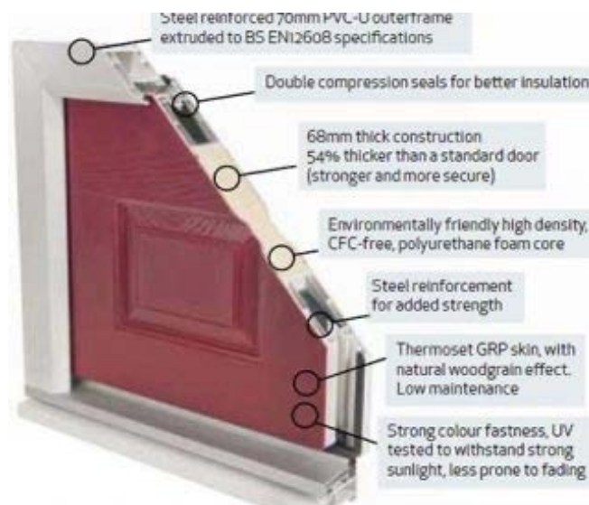
Composition of composite doors (using steel reinforcement)
