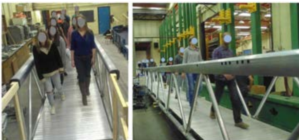
Crowd tests on an aluminium bridge to assess excessive vibration response 8
