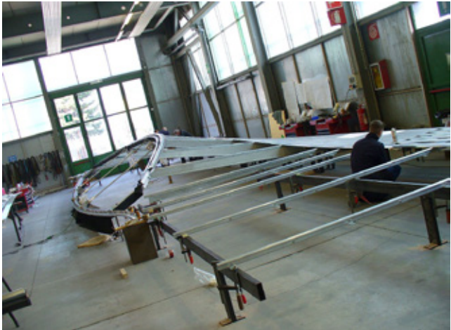
Fig 4.33 Façade prototype of an 'eye lid' or sky window and aluminium cladding being assembled in Frener & Reifer's workshop
