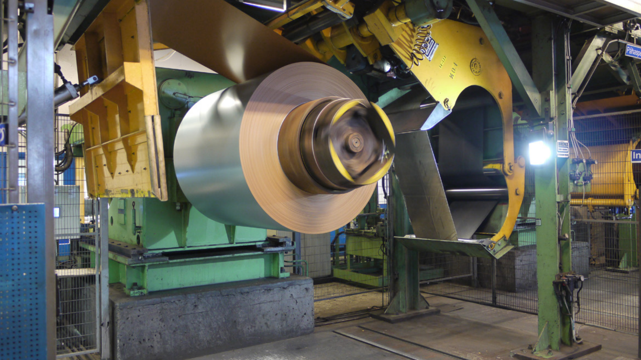
Fig 2.38 A primed coil of aluminium entering Hydro's automated coil coating line in Holmestrand
