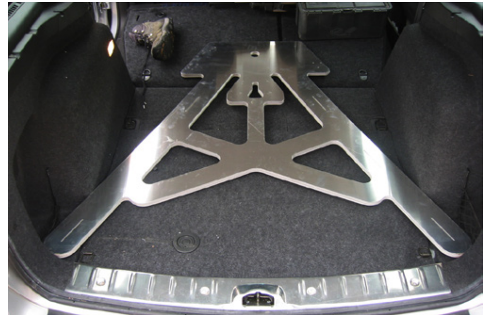
Fig 2.118 The prefabricated aluminium components are sized for transportation in the architect's car
