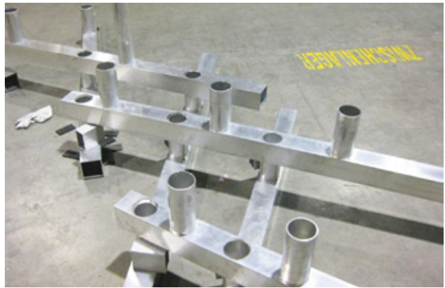
Fig 5.218 The structure is formed from standard extruded aluminium box sections linked by tubular aluminium sections
