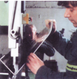
Fig 2.49 Aluminium gutter of East Croydon Station being press braked by Majors of Croydon
