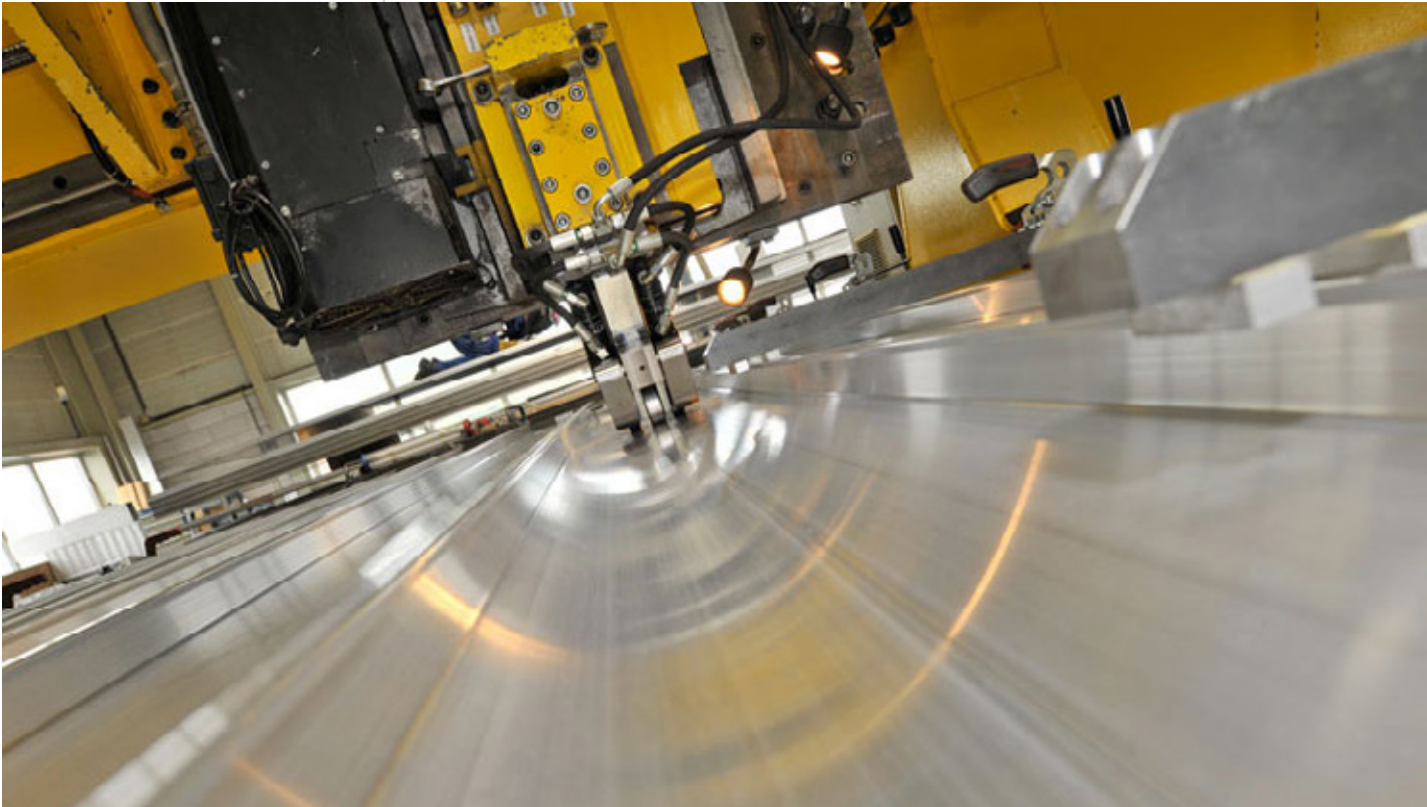
Fig 10.14 Friction stir welding, the bottom tray of the Large Hadron Collider at Bayards
