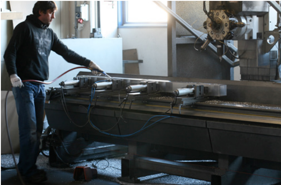
Fig 2.81 Machining a circular port in a square extruded aluminium section during the fabrication of Vague Formation
