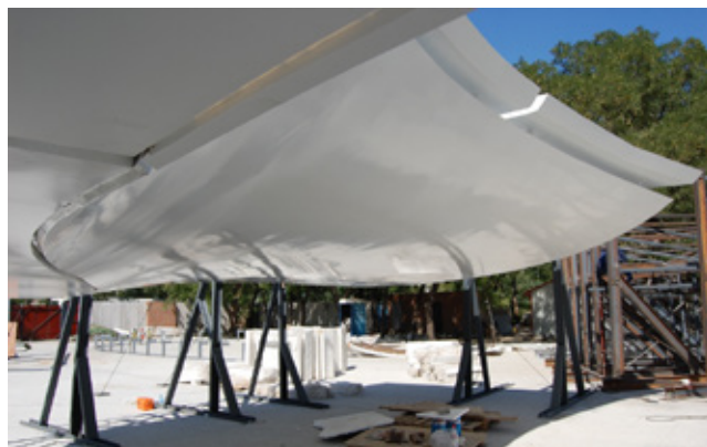
Fig 9.48 The 3mm polyester powder coated aluminium of the prototype fabricated by Permasteelisa
