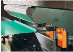
Fig 2.44 Press Braking a 90° edge, a second 90° is about to be formed (photograph courtesy of ame)
