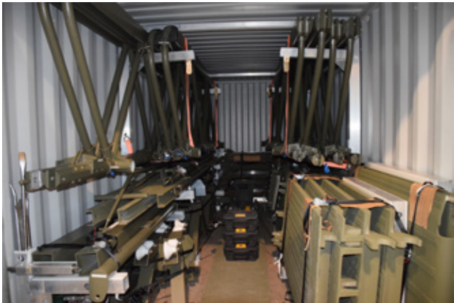
Fig 5.103 Inside a 6.1m container all the components of the prototype bridge
