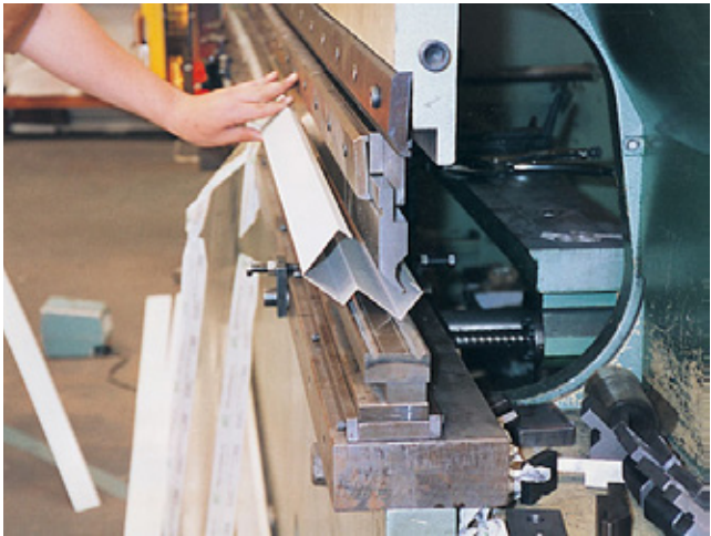
Fig 2.48 It is essential to design for removal from the press tool
