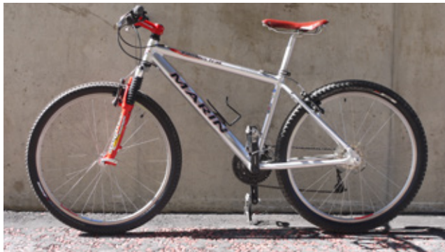
Fig 2.11 The author's twenty year old Marin mountain bike with a welded 7005 aluminium alloy frame and new British leather saddle
