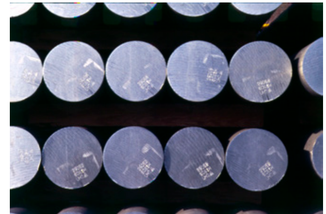
Fig 2.160 Aluminium billets waiting to be extruded at Joseph Gartner's works, note the alloy code is stamped on each billet
