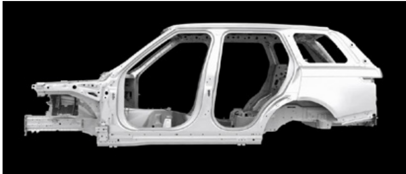
Fig 1.28 The Range Rover 2013 – a mimetic design that is 420kg lighter than the previous model
