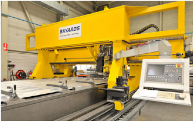
Fig 10.15 Friction stir welding machine at Bayards
