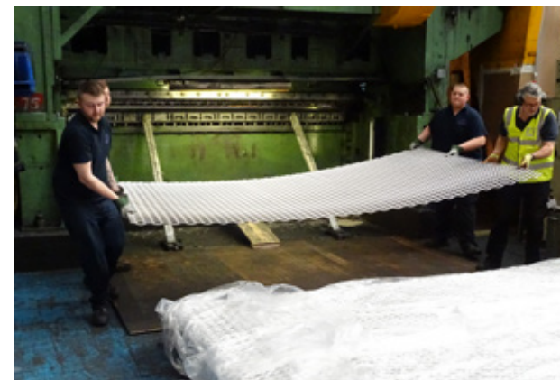
Fig 7.37 Each sheet of expanded aluminium is light enough to be easily carried by four people
