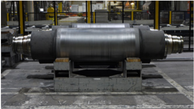
Fig 2.26 Work rolls from Hydro's hot rolling line, Holmestrand, Norway
