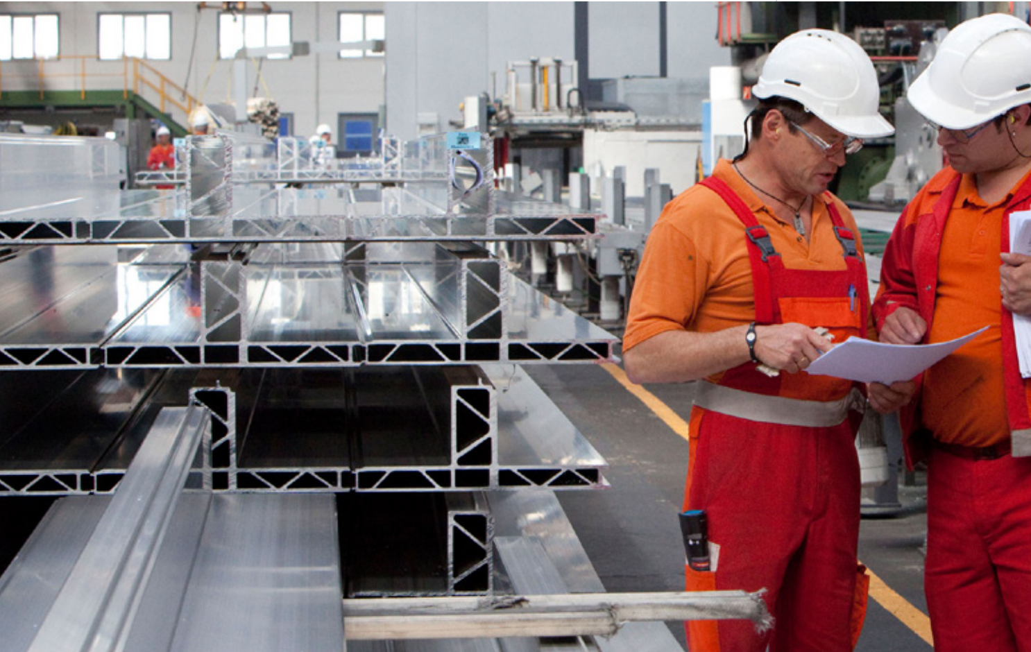
Fig 1.5 Large format aluminium alloy extrusions in Constellium's plant, Singen, Germany
