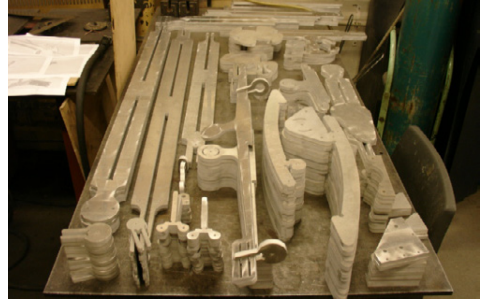
Fig 2.117 The waterjet cut aluminium components of Kielder Probes
