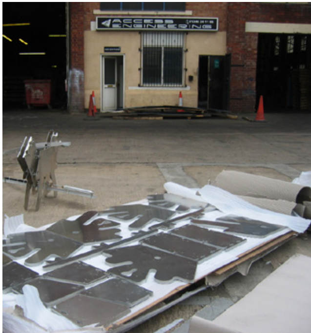
Fig 2.116 Impromptu trial assembly outside Access Engineering who waterjet cut the components
