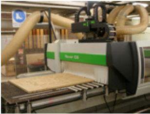
Fig 2.63 CNC machining of MDF components
