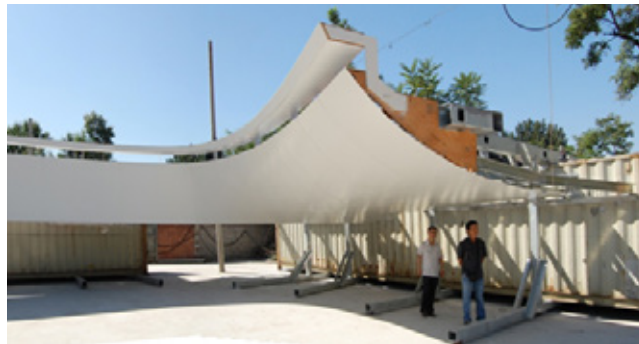
Fig 9.47 The first prototype fabricated by Permasteelisa in October 2009 from 3mm polyester powder coated aluminium
