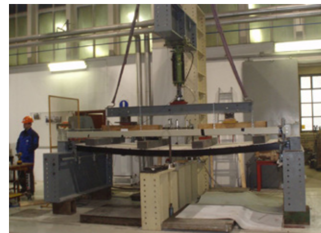
Fig 7.4 Load testing of a QbissAir façade panel
