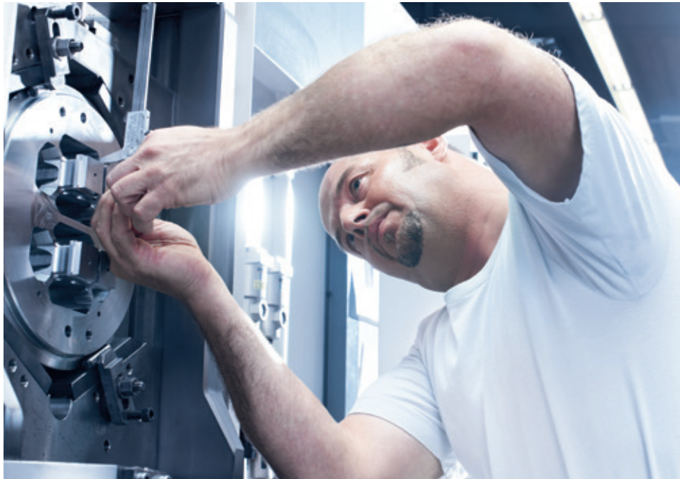
Fig 2.161 A die maker from Wefa installing a porthole die for extruding a hollow aluminium section
