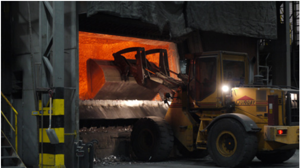
Fig 2.21 Post consumer aluminium scrap from the United Kingdom being loaded into the furnace of Hydro's cast house, Holmestrand, Norway
