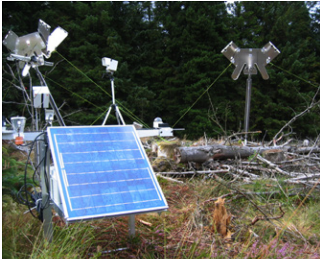
Fig 2.121 The Probes are monitoring and responding to the environment, opening out when warm and sunny, closing down when cold and dark
