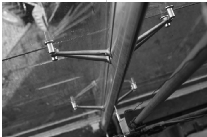
Fig 2.173 Extruded aluminium mullion, stainless steel castings and 10mm toughened glass wall assembly of East Croydon Station being weather tested at Taywood Engineering
