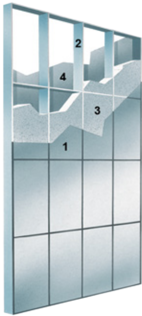
Fig 3.60 Kalwall panel module: 1 Translucent glass fibre reinforced polymer (GFRP) exterior face 2 Structural Grid Core (aluminium extrusion or thermally-broken aluminium extrusions) 3 Translucent insulation (TI) thermal packages including aerogel 4 Translucent glass fibre reinforced polymer (GFRP) interior face
