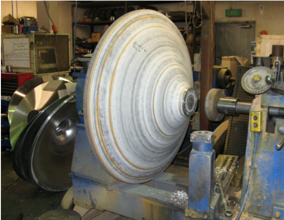
Fig 2.51 A metal spinning tool
