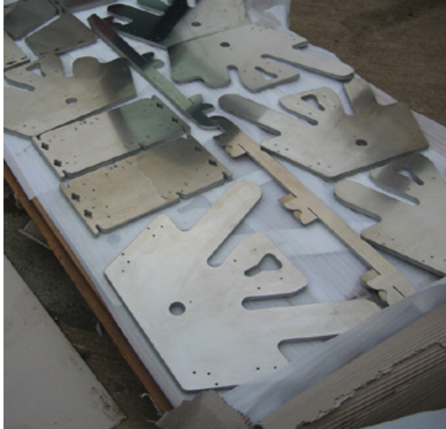
Fig 2.115 Waterjet cut components of Kielder Probes
