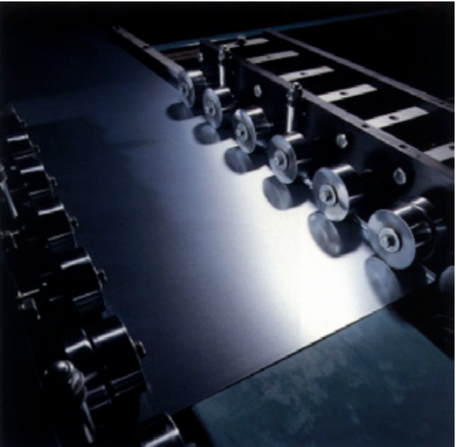
Fig 2.41 Roll forming the edges of a metal sheet to form the face of a metal composite panel
