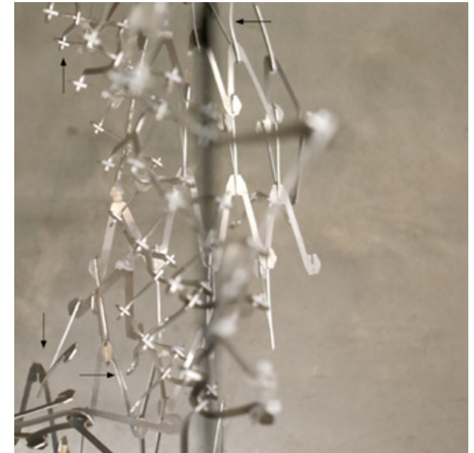
Fig 2.106 [right] The third assembly of the Protocell Mesh, some aluminium components show a need for greater robustness in repeated assembly and disassembly
