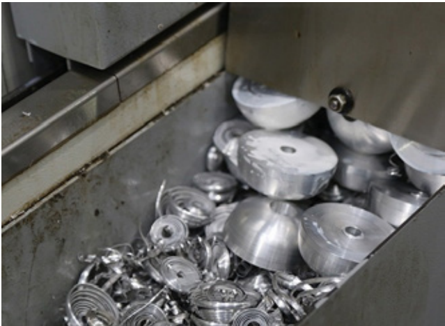
Fig 2.134 Machined aluminium alloy nodes of the Hive, in Stage One's Workshop
