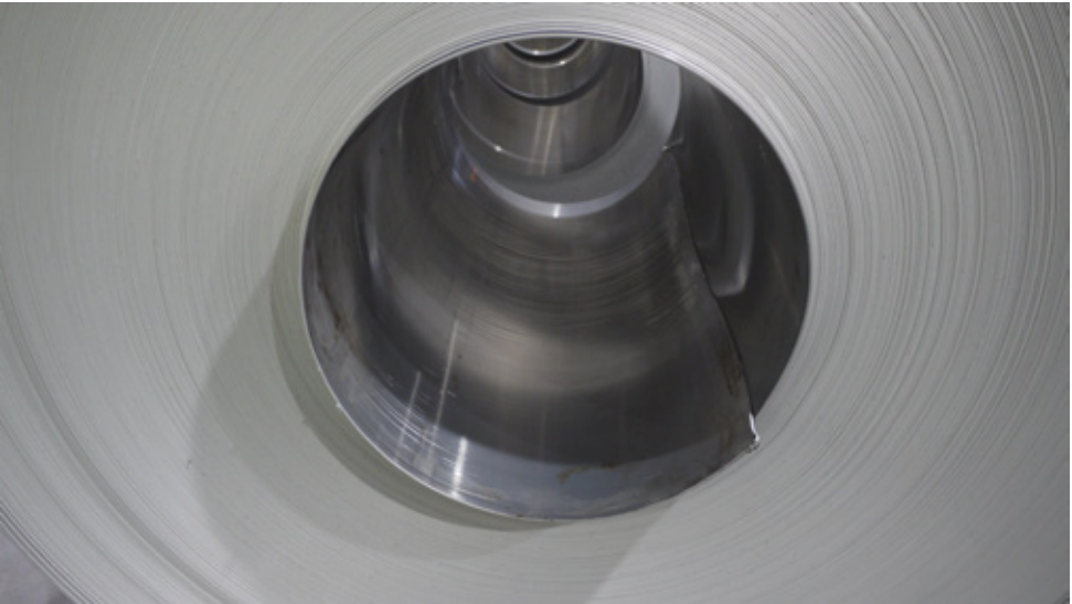
Fig 2.27 A 7 tonne coil of hot rolled aluminium
