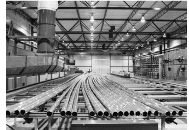
Fig 2.159 Extruded aluminium tubular sections, before straightening, at Sapa Tibshelf Plant, Derbyshire, England, design by Foster Associates, 1973
