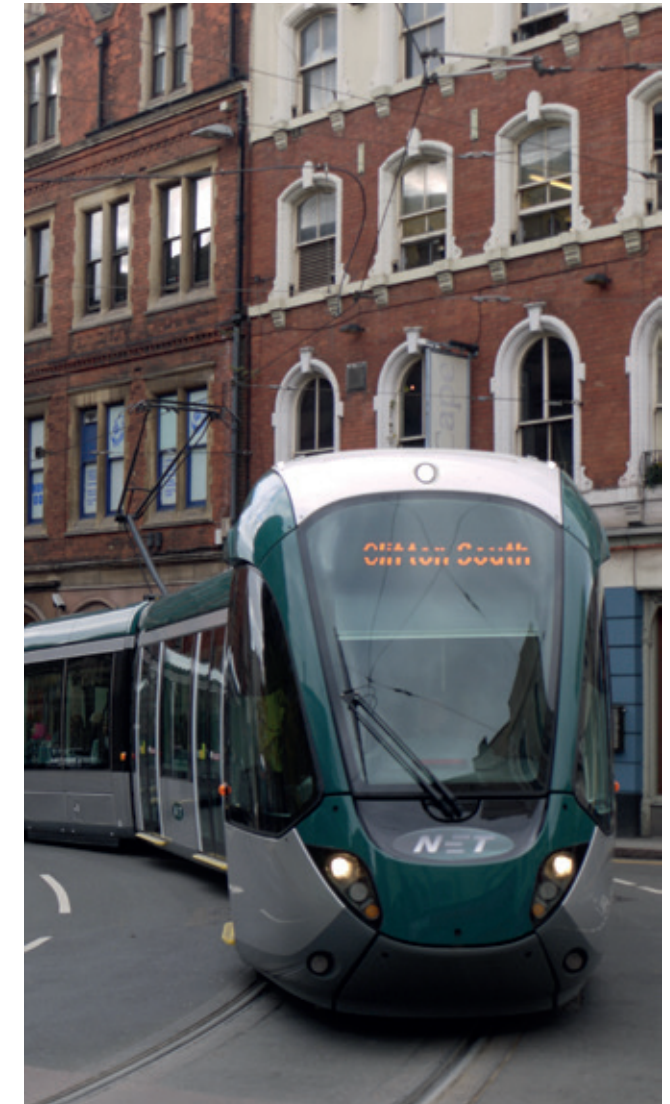
Fig 1.26 A Nottingham NET Citadis 302 tram built by Alstom in 2014, with an all aluminium body
