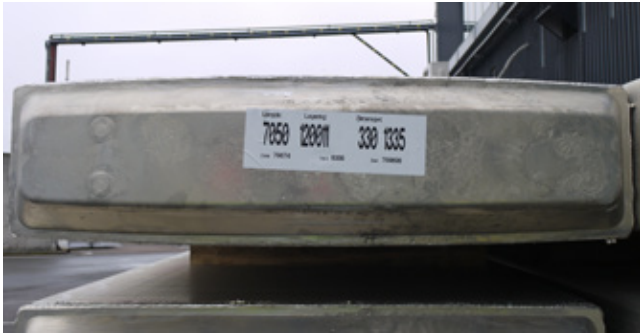
Fig 2.22 A 7 tonne cast aluminium ingot of 1200 alloy outside Hydro's hot rolling line, Holmestrand, Norway
