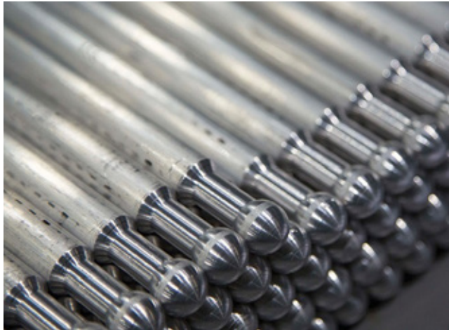
Fig 2.138 Machined ends of the aluminium connection rods
