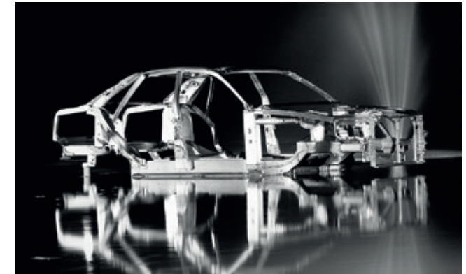
Fig 2.5 Audi's welded aluminium space frame of the Audi A8
