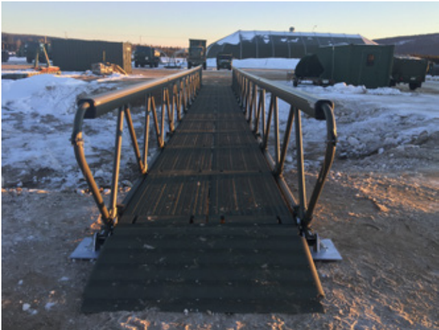
Fig 5.102 Rapidly deployable military bridge on test by the Canadian Army
