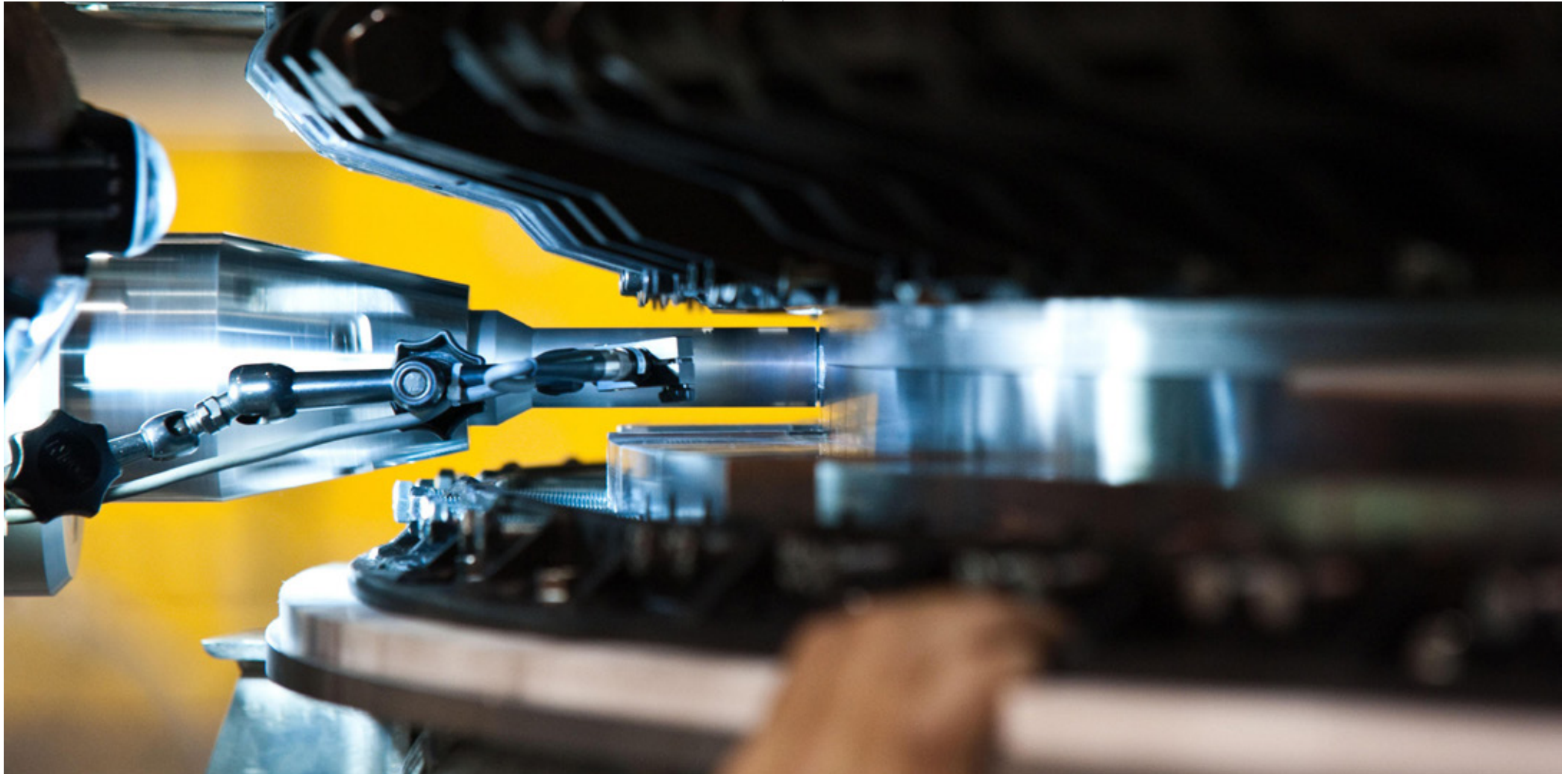
Fig 2.152 The bulkhead and nosecone of the Orion spacecraft are joined using friction stir welding, courtesy of NASA
