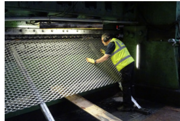
Fig 7.35 The expanded aluminium sheet being manufactured in Hartlepool
