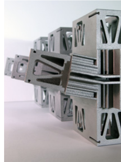
Fig 2.154 Digitally printed aluminium Nematox II nodes
