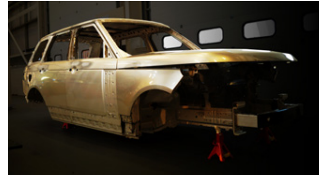
Fig 1.30 A prototype all aluminium alloy body shell of the Range Rover 2013 at Rover 2012 Prototyping Architecture, Nottingham
