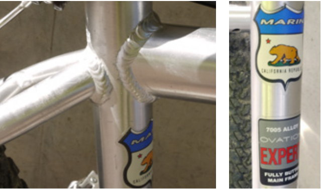
Fig 2.19 Precise yet visible welding of the frame of a Marin mountain bike
