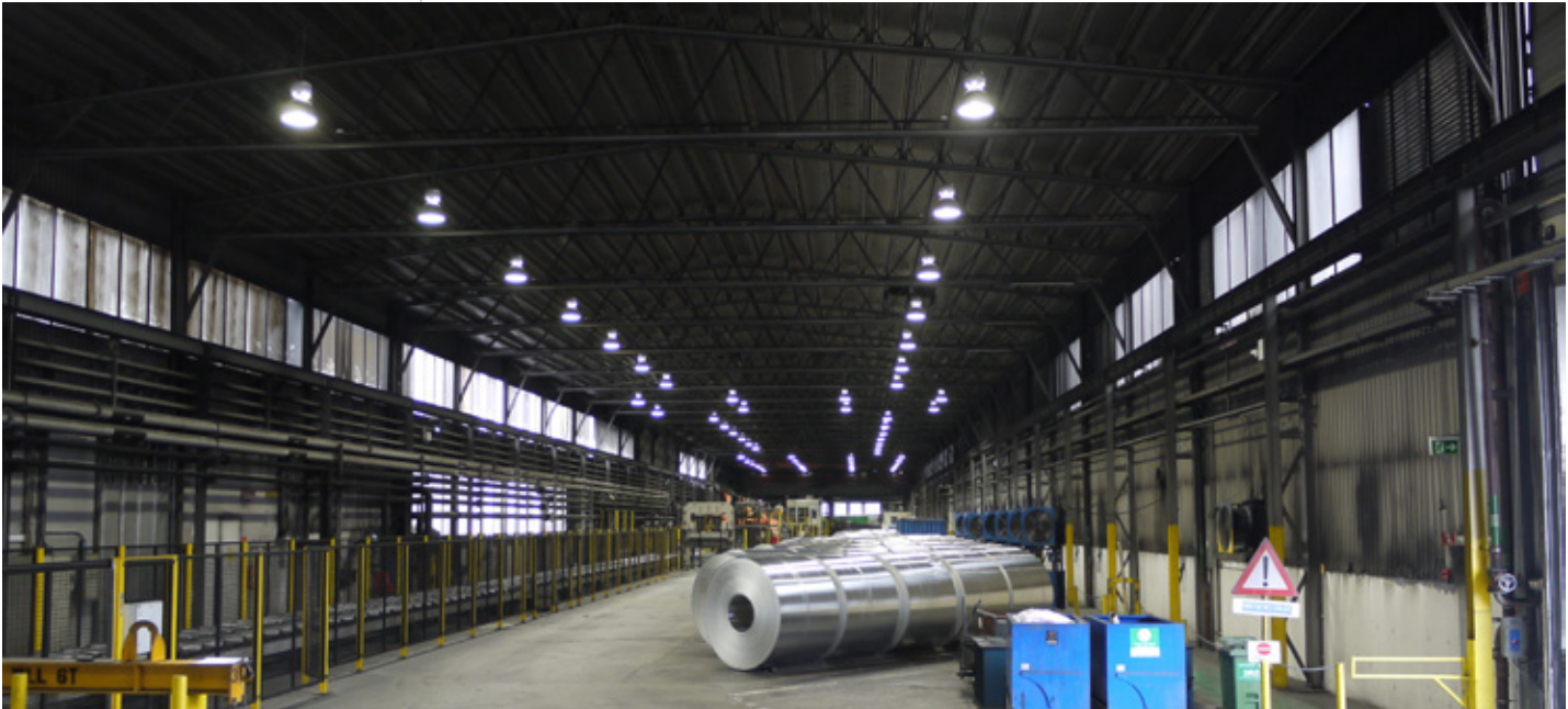
Fig 2.28 Coils of hot rolled aluminium cooling next to Hydro's hot rolling line, Holmestrand, Norway
