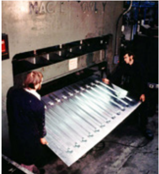
Fig 5.29 Pressing aluminium cladding panels at Kinain Workshops
