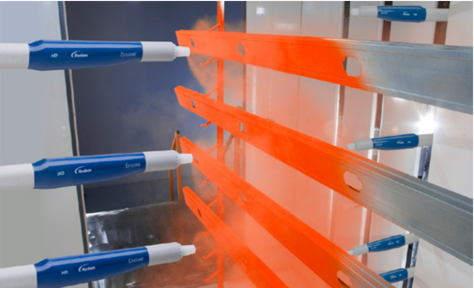
Fig 2.4 Electrostatic application of polyester powder coating, courtesy of Nordson
