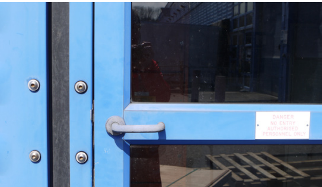
Fig 5.32 Hewi nylon-coated door handle significantly eroded down to its metal core
