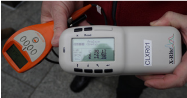
Fig 6.3 DFT meter used to measure coating thickness and X-Rite colour meter
