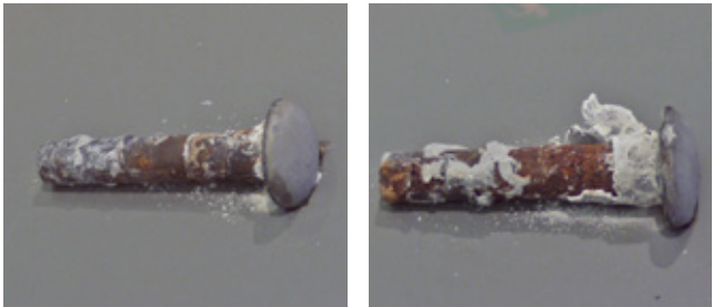
Fig 4.20 [left] Aluminium-capped bolts showing the longevity of aluminium compared to the rusted steel
