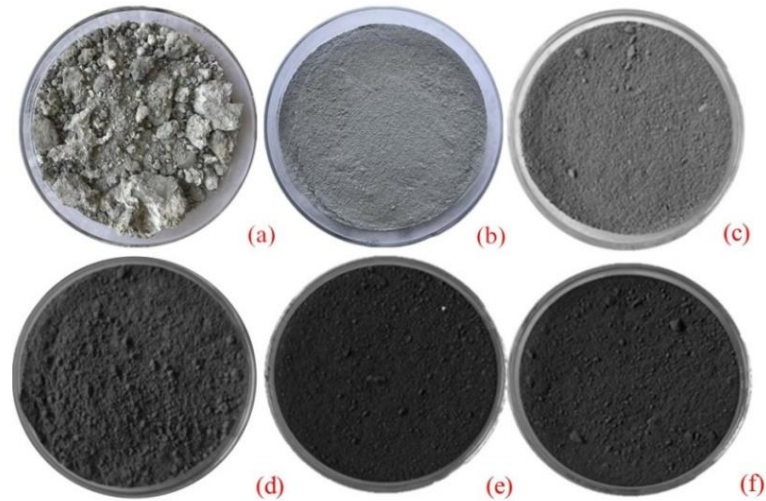
Figure 2-1 Aluminum slag and secondary aluminum dross from different sources (a) Primary Aluminum Slag from Henan (b) Primary Aluminum Dross from Henan (c) Primary Aluminum Dross from Guangxi (d) Aluminum Alloy Dross from Jiangsu (e) Aluminum Alloy Dross from Hebei (f) Aluminum Recycled Dross from Jiangsu
