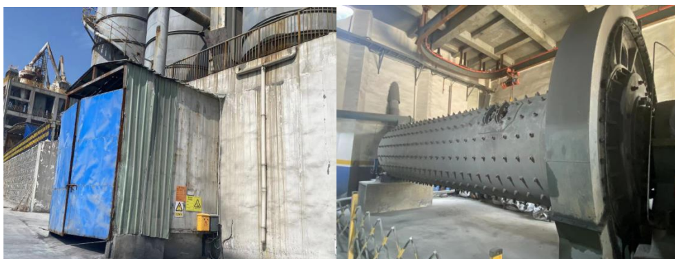
Figure 4-4 Secondary aluminum dross discharge and ball mill for mixing and grinding
