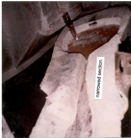
Figure 109: Boron treatment conducted in the launder for neutralizing negative effect of V on conductivity of the product [252].
