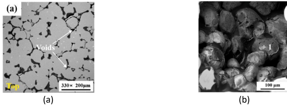
Figure 69: Purified aluminium alloys: (a) polished sections; (b) collected aluminium particles. Reproduced from Sun et al.[148].
