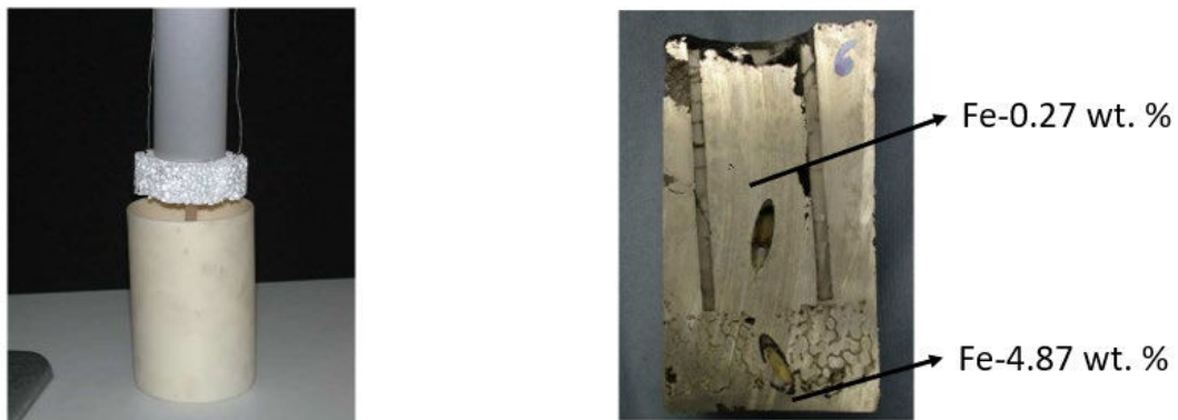
Figure 48: laboratory design of forced filtration set-up: (a) snapshot; (b) result of proof-of-concept test. Reproduced from [102].
