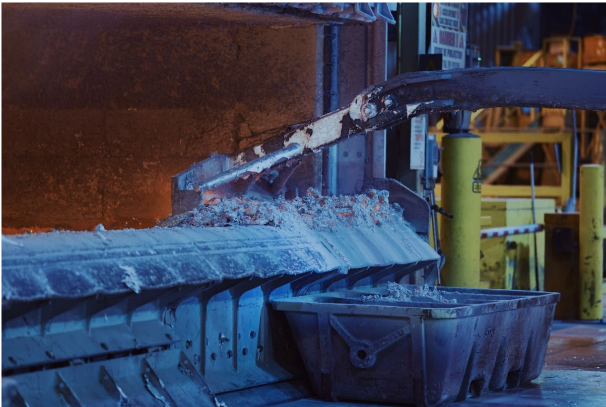
Figure 18: Skimming of the dross out of furnace into dross pan. Photo: Courtesy of Rio Tinto
